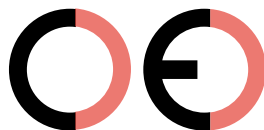
False CE Mark (too far)
